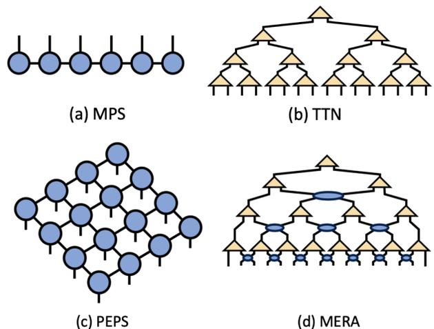
FIG. 8. Different types of tensor network simulators: (a) Matrix Product States (MPS), (b) Tree Tensor Networks (TTN), (c) Projected Entangled Pair States (PEPS), and (d) Multi-scale Entanglement Renormalization Ansatz (MERA).
