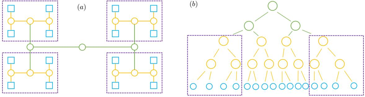
FIG. 3. (a) Self-similar fractal structure of the H-tree designs (see [273]). One can use the self-similar structure to create a size  $2^{n+2}$  QRAM from 4 units of size  $2^n$  QRAM. (b): An example of depth-4 tree with  $2^4 = 16$  leaves.
