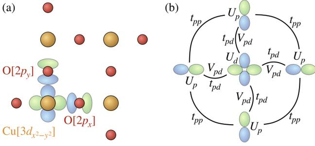
FIG. 12. (a) schematic view of a  $[\text{CuO}_2]_4$  cell in a cuprate  $\text{CuO}_2$  plane. Cu/O atoms are represented with orange/red circles and orbitals by blue and green contour plots (blue/green for positive/negative values). (b) definition of the three-band Hubbard model parameters (the curve connectors represent the kinetic energy coefficients).
