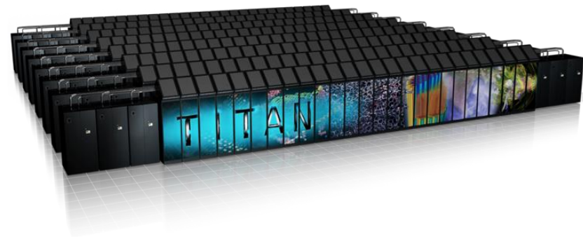
Cray XK7, 18,688 Nodes 16-core AMD Interlagos + K20X 17 PFLOPS, 8.2 MW, #1 TOP500 (2012)
